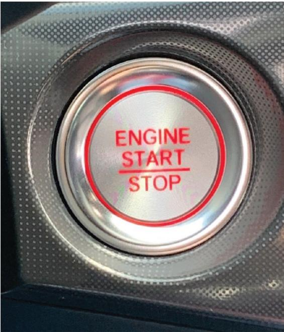
3. Start the engine by pressing the ENGINE START/STOP button while pressing the clutch pedal and brake. You must start the engine within **10 seconds** of touching the remote to the button.
