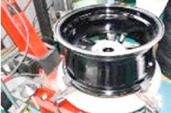
Before changing the tire, attach a protector to each changer clamp to prevent damage.
