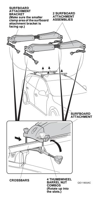
3. Secure the surfboard attachment by tightening the two thumbwheels evenly as shown. Repeat for the remaining six thumbwheels.
