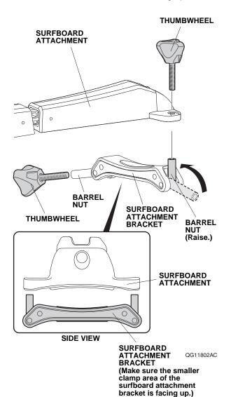
Install the surfboard attachment assemblies on the crossbars with the brackets around the crossbars.
