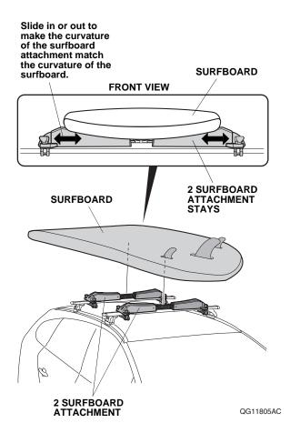
5. Secure the surfboard attachment by tightening the two thumbwheels evenly as shown. Repeat for the remaining six thumbwheels.
