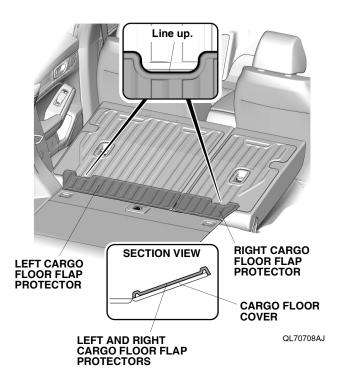
7. Secure the left and right cargo floor flap protectors.
