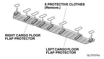
6. Position the left and right cargo floor flap protectors.
