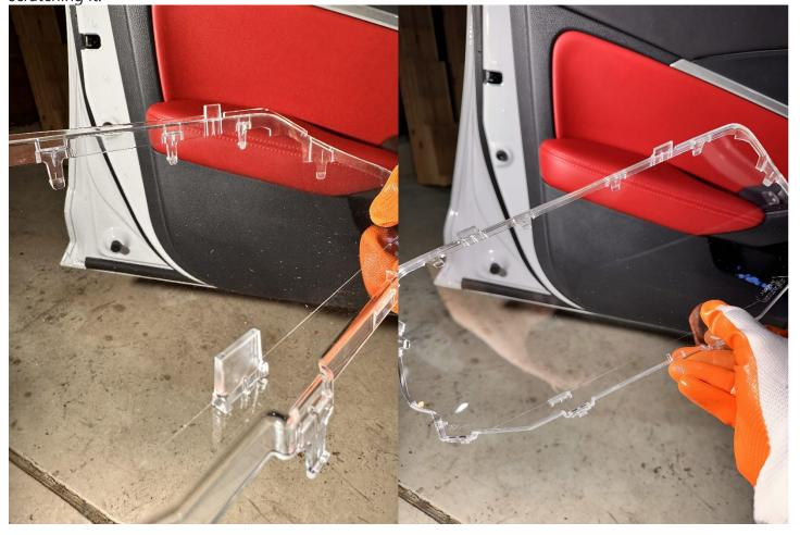
**Step 11:** Transfer the **four rubber pieces** from the old lens onto your new lens. These help seat the **bezel**
