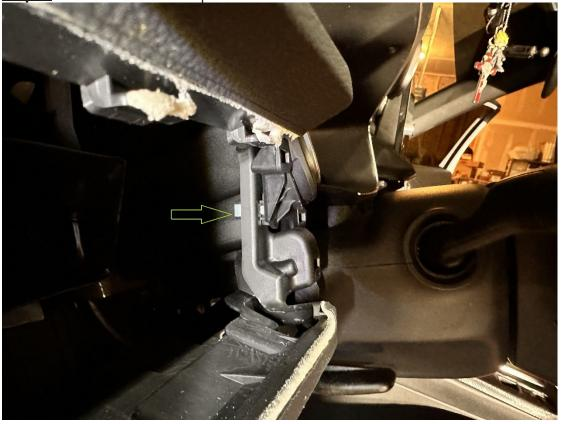
**Step 4:** be careful not to break the tabs noted from the blue arrows. If these break the entire vent will move around and rattle. I've also added some insulating tape to help eliminate rattles from plastic
