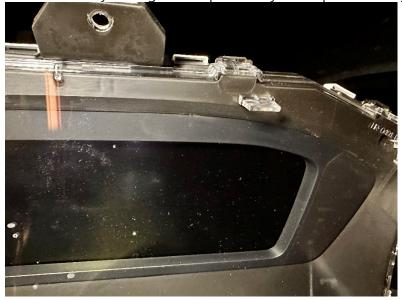
**Step 10 [Optional]:** The new lens has brand new PPF already installed. I added ceramic cover over it a day prior. This step is optional. I did this to freely wipe down the new lens in the future without worrying about scratching it.
