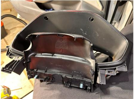
**Step 8:** Remove three scrips in the yellow circles with Phillips screwdriver. Using your fingers or a flathead screwdriver, press down and pull apart all the tabs at the green arrows.
