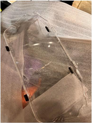
**Step 12:** Pull apart the old lens and fasten the new lens onto the **digital gauge cluster**. The eight tabs snap in fairly easily.
