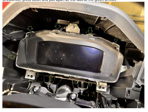
**Step9:** Once all retaining tabs are loosened, DO NOT completely pull apart yet. Get the replacement lens ready for immediate installation as to not allow dust particles to get inside. I had my toddler hold a vacuum nearby during this step for stray dust specs floating around.
