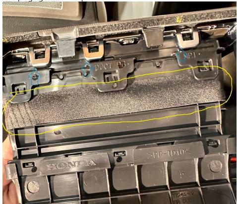
**Step 5:** Remove two screws with a Phillips screwdriver to detach the **gauge cluster bezel**
