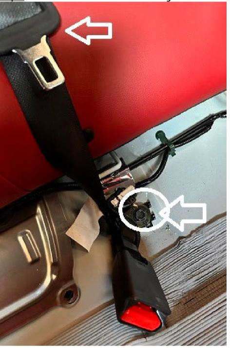
Step 9: Install the new seat bench assembly and clip both U-brackets onto the white clips. Then pull all
