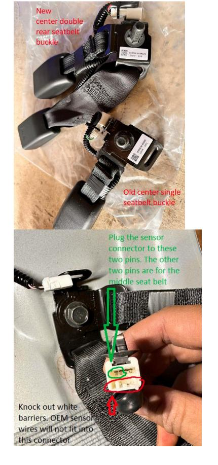
Note: Turn car on with seatbelt attached to the buckle to verify you've selected the correct pins
