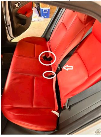
Step 10: Reinstall the retaining bolt to attach the seat bench assembly to the frame
